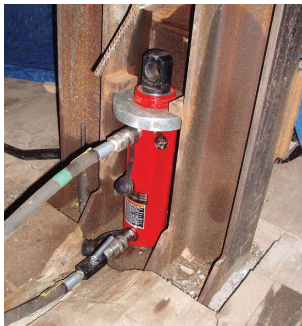
HD cylinders can be used in pushing and pulling applications. In this photo, we see a HD2506 HD cylinder set up for a pull application using a Plunger Clevis cylinder accessory
